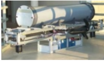
Figure 1 – A forward/side view of the vehicle. Note the aluminum thermal endcap.
